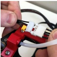
Connect the extruder motor with the provided custom extension cord
