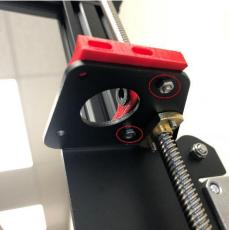
Install the filament guide bracket using provided M3 bolts and nuts
